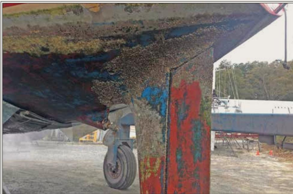
**For close to a year, *Gypsy Wind* went without bottom paint, the only protection came from the Ultrasonic unit. Once hauled, the exposed layers of old bottom paint, offering no antifouling protection, were visible (top). The only significant area of barnacle growth after this extended period was near the skeg (bottom).**
